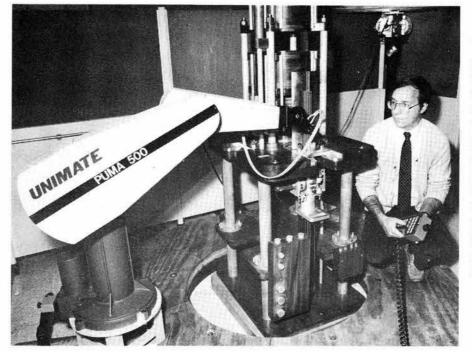
"SIT" is the electronic command that Jim Banas seems to be giving the robot. Actually, his group is programming the loon-lookalike machine to perform maintenance operations on SPR-III—a Sandia-operated DOE reactor. Jim is the head of Intelligent Machine Division 6228, which was recently created to pursue the technology of intelligent machines as it relates to Sandia programs.
